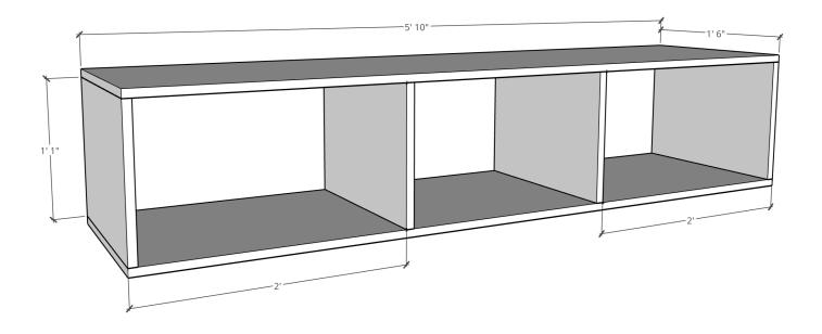
The case for this cabinet is made from 3/4" plywood and uses butt joints reinforced with glues and screws. The carcas is really easy to make, it's just a box that is 70"x14.5"
